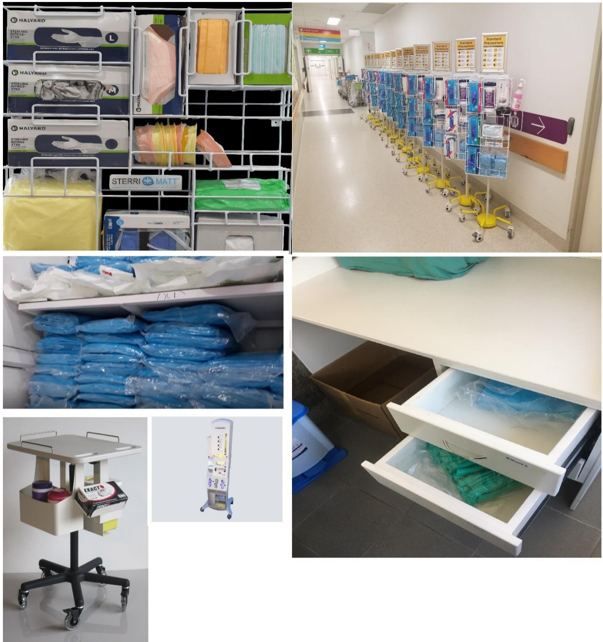
Figure 10: PPE stations / dispensers / organizers are necessary at donning stations. These can range from being sophisticated to being simple drawers. Regardless, hiding PPE inside locked cupboards, while it can prevent abuse, will also lead to under-use and therefore will increase the risk of cross-contamination. Some of the pictures are from the public hospitals of Mauritius. See references 11-14 for details.
