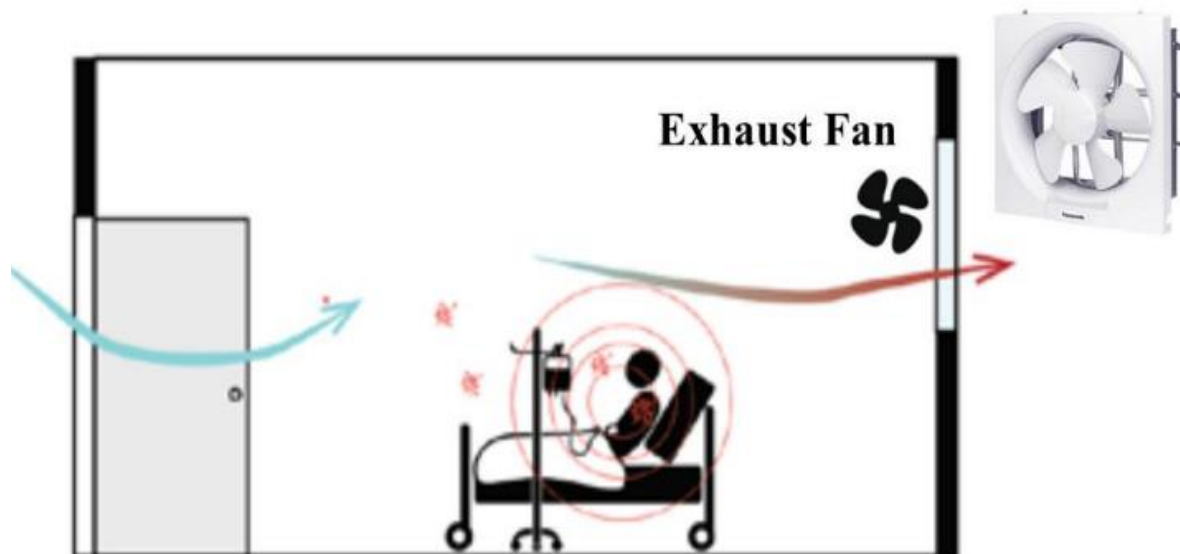
Figure 21: Cross-ventilation is better than single-sided ventilation; however, doors to corridors cannot be left open if the patient is suffering from an airborne illness. Use fans or air extractors to ensure that the air is pulled out of the facility and not pushed inside. Split air and ductless air conditioners should be turned off. See reference 2 for details.
