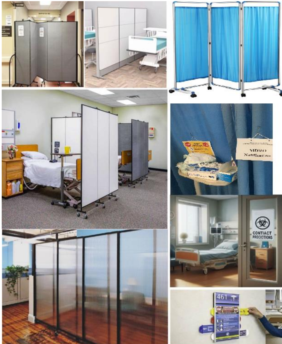
Figure 11: Cubicle dividers do not need to be made of aluminum, reach the ceiling or be bulky – these can reduce ventilation and make it difficult to maneuver around patients. Practical alternatives are shown above – they are cheap, mobile and can be made of plywood, glass or plastic. They can be transparent or not. They need to be high enough to be above the nose and should be more than 1.2m tall. The importance of these barriers for patients requiring contact or droplet precautions is mostly to allow signages to be displayed so that appropriate precautions are taken when coming close to the patient. If cloth curtains are used, they need to be sent for laundering during terminal cleaning. The second picture on the right column from top to bottom is from Dr A. G. Jeetoo Hospital. See references 15-17 for details.
