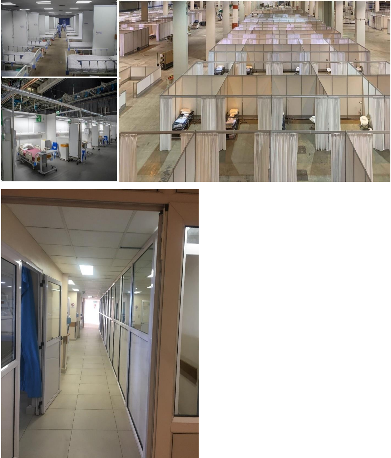
Figure 6: Single en-suite rooms are often not required for patients needing contact or droplet precautions. Simple washable dividers can be placed in between patients and are often cost-effective. Commodes or bedpans should be used; if this is not possible, common bathrooms need to be cleaned more often. The bottom picture is from Dr A. G. Jeetoo Hospital. See references 4-6 for details.
