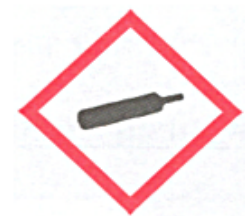
Gas under pressure
